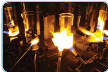
Because of the higher melting point, more heat and labor are required to produce borosilicate glass. The benefits of borosilicate glass far outweigh the additional cost to manufacture.
