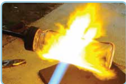
Used for glass blowing and lampworking, borosilicate glass has a higher melting point, able to withstand a wide range of temperature changes without cracking or shattering.
