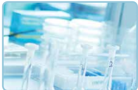
Borosilicate glass is used for scientific laboratory and medical equipment because of its clarity, temperature and chemical resistance.
